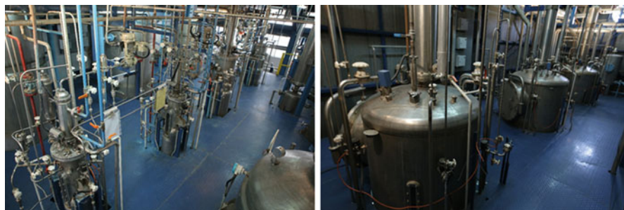
Fig. 10.5 The fermenters of the Nature Biotechnology Company, Biorun, for microbial control agents' production
