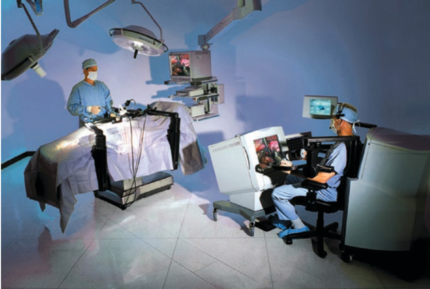
Fig. 2 ZEUS:First clinically used robotic-system for laparoscopic coronary artery revascularization. Open console, instruments with only 5 degrees of freedom (DOF). 3D-Video-technology using a helmet with two screens or only 2D-videotechnology
