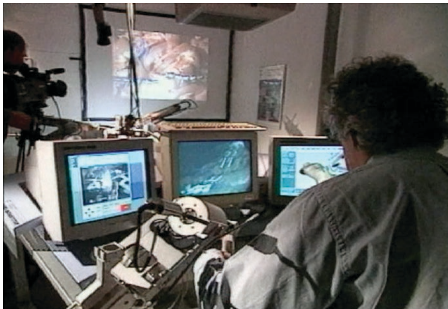
Fig. 1 ARTEMIS: First master-slave system used experimentally (G. Buess, German Nuclear Research Centre, Karlsruhe, Germany). Open console, 3D-videotechnology with polarizing glasses for the surgeon
