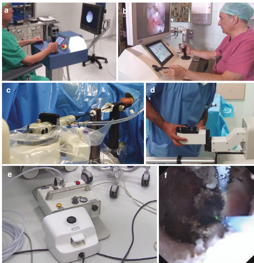
Fig. 7 Avicenna Roboflex System (ELMED, Ankara, Turkey): (a) Prototype with non-ergonomic handles and small screen, (b) Open console with sophisticated left-hand joystick for rotation and insertion/retraction and fine-tuned right-hand wheel for deflection. Touchscreen functions for laser activation, irrigation, and fine-tuning of movements, (c) Robotic arm with the hand-piece of a digital flexible ureteroscope (Flex XC, Karl Storz, Tuttlingen, Germany) fixed in the master plate and the flexible part supported by one or two stabilizers before entering the access sheath, (d) Exchange of the master-plate (i.e. when using a disposable device), (e) Pneumatic driven device for activation of the laser foot-pedal, (f) Endoscopic image of robot-assisted Thulium-laser ablation of upper tract urothelial carcinoma (single-kidney)
