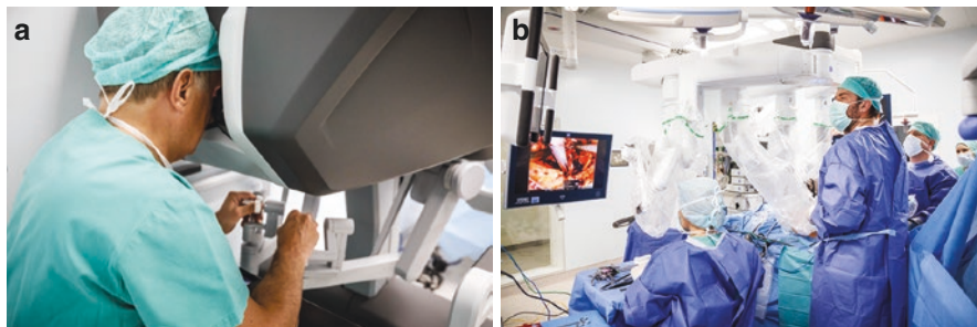
Fig. 4 DA VINCI XI: Console of last generation of robotic system for interdisciplinary use (a) In-line view with 3D-HD-videotechnology, 7 DOF for all instruments. Four-arm-system, telescope can be inserted via every port access. OR-table (Trumpf-Medical) can be moved without undocking of the robot
