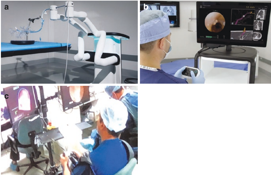
Fig. 6 Monarch (Auris Health, Redwood City, CA, United States): (a) Robot for flexible endoscopy designed for bronchoscopy. Two-arm-system for control of inner and outer sheath. Optional third arm for percutaneous access, (b) Movement of the robot is controlled by a handheld keypad like for computer games, (c) Experimental use of the device with a single-use robotic ureteroscope
