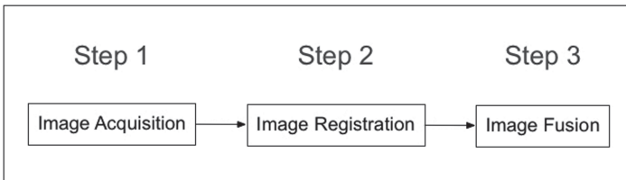
Fig. 1. The framework of image processing
