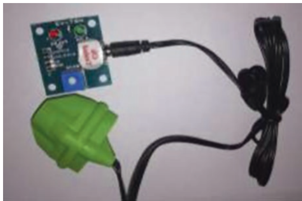
Fig. 12.2 Heartbeat pulse rate sensor
