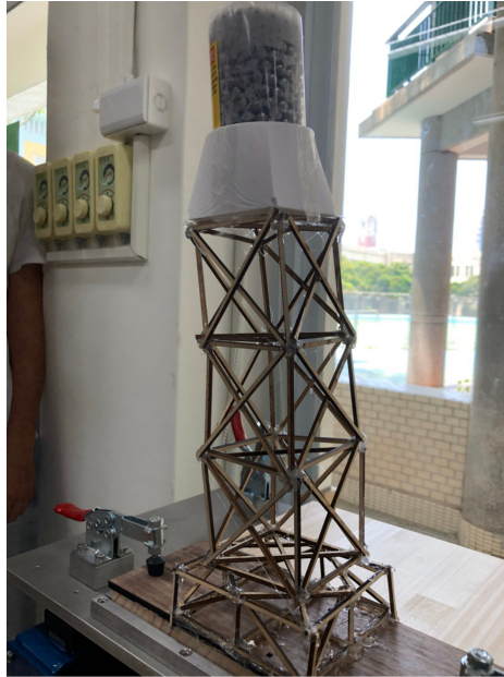
Fig. 3. Water tower truss structure
