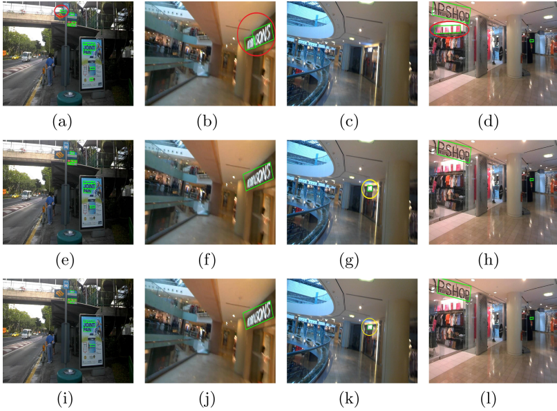
Fig. 4. Detection results from EAST+CBCE , EAST+CBSAL and EAST+CBFPL : (a)–(d) from EAST+CBCE ( Baseline ), (e)–(h) from EAST+CBSAL and (i)–(l) from EAST+CBFPL . The boxes in red ellipses represents wrong results while other boxes are correct. (Color figure online)
