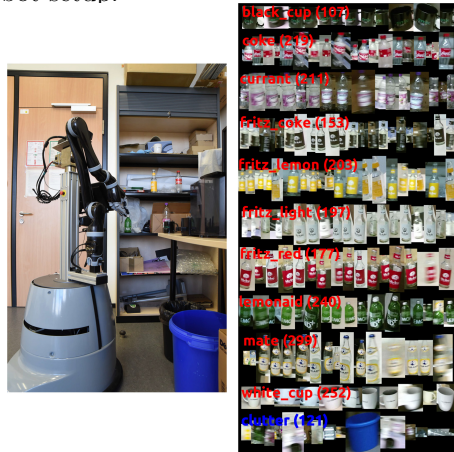
Fig. 4. Left: Our service robot capturing objects in a cluttered shelf. Right: Some class representatives from our recorded real world object data set CUPSNBOTTLES. The number of a class's object samples is given in brackets.
