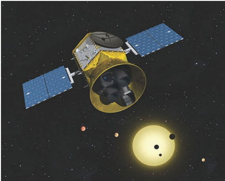
Fig. 10.6 Artist concept of the transiting exoplanet survey satellite and its 4 telescopes. Credit: NASA/MIT
