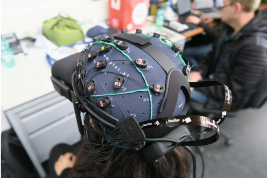
Fig. 6.4 The 32 electrodes EEG device used in COGITO in space. Photo: Sandro Bocci, 2017
