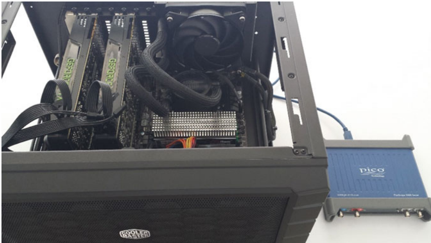
Fig. 7.10 Picture of the internals of the first final spectrometer. Inside the PC case, on the left, the GTX 680 GPUs, in the center the memory and the liquid-cooled CPU, outside the new Picoscope DAQ
