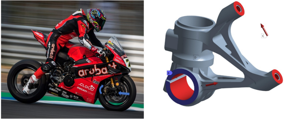
Fig. 5. Load and constraints on the front wheel support
