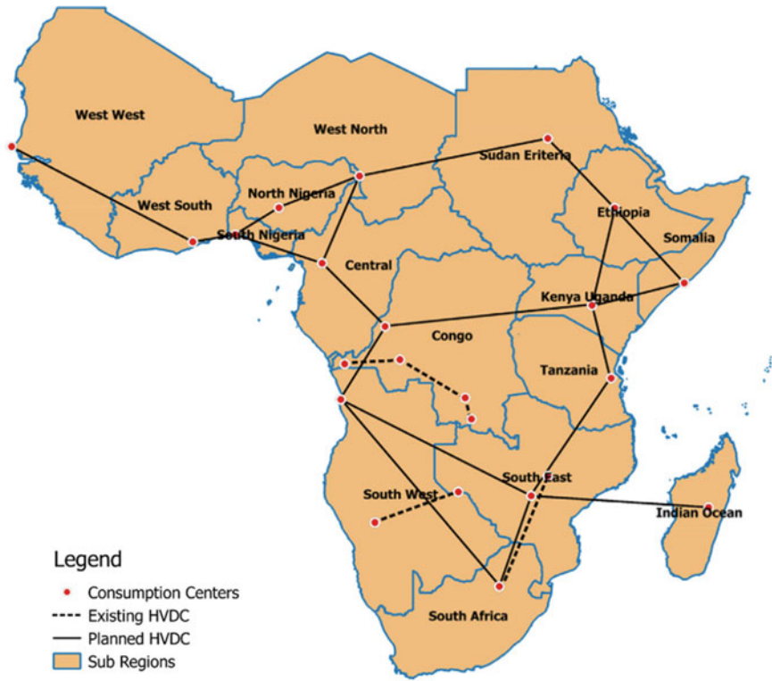
Fig. 7 SSA Sub-region transmission line configuration [7]
