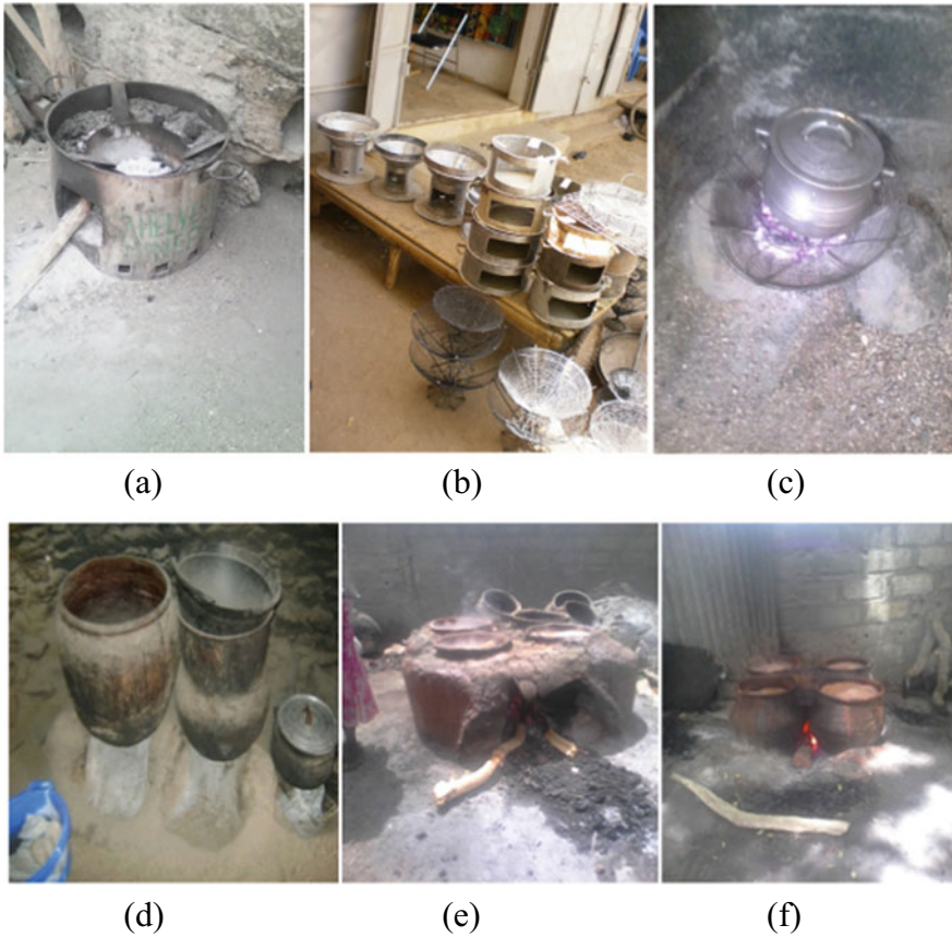
Fig. 3 Some of the biomass stoves used in Cameroon. a, b Metallic stoves, c wire grate charcoal stove, d, f improved three stone stove (All pictures by Viyoi Catherine TANGKA reproduced with permission from Viyoi [21])
