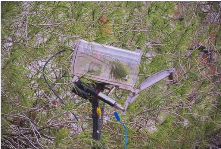
Fig. 14.4 Chambers used for shoot-scale CO 2 and water flux measurements in Yatir Forest
