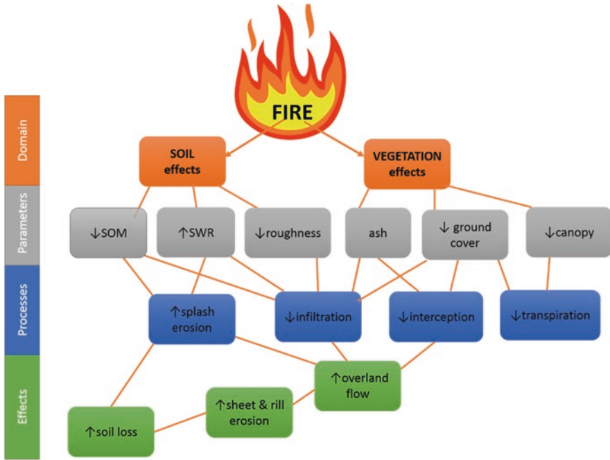
Fig. 23.2 Domains of fire effects on soil erosion: parameters, processes and net effects
