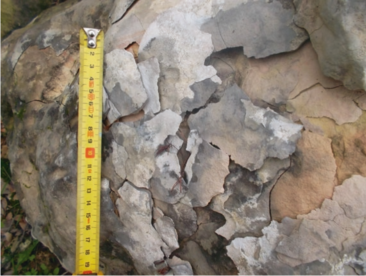
Fig. 23.1 Burned rock spalling, Arqan Formation, 2010 fire Mt. Carmel. (Photo: Nurit Shtober-Zisu 10/12/2010)
