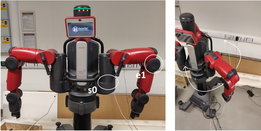
Fig. 1. A pair of images of the Baxter Robot. The left image shows the whole robot, the controlled joint ( s_0 ) and the location that was being controlled ( e_1 ) through moving s_0 . The right image shows the effect of applying force to the s_0 joint, either positive or negative.
