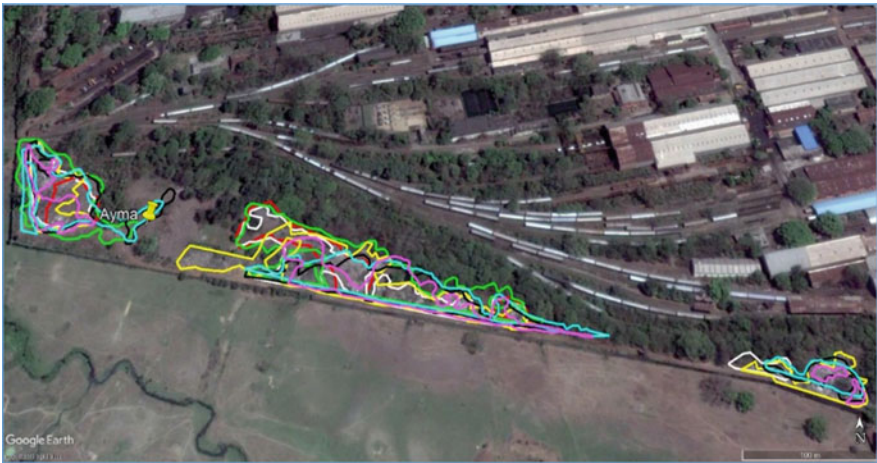
Fig. 9.3 Time-series analysis of Ayma dumpsite (colour code: Red, 13-Jan-2011; white, 20-May-2012; green, 19-Apr-2013; yellow, 30-Mar-2014; black, 22-Nov-2015; cyan, 29-Mar-2016; pink, 30-Oct-2016)
