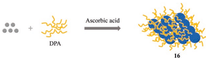
Fig. 3.8 Synthetic strategy of AIE-based Cu NPs 16 . Red-emitting 16 was prepared by using DPA as a stabilizing agent and ascorbic acid as reductant. Adapted from Lin et al. (2016) with permission from Elsevier
