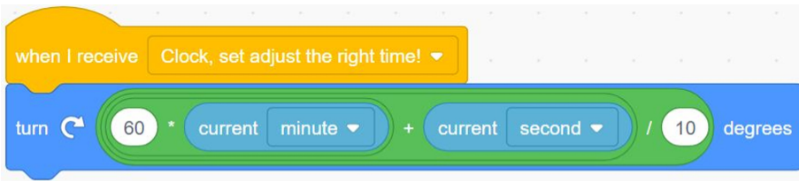
Fig. 2. Example of mathematical description of the circular motion of a big (Minute) hand clock
