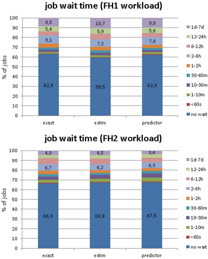
Fig. 6. Distribution of job wait times with respect to the walltime being used (exact runtime, user estimate, predictor).
