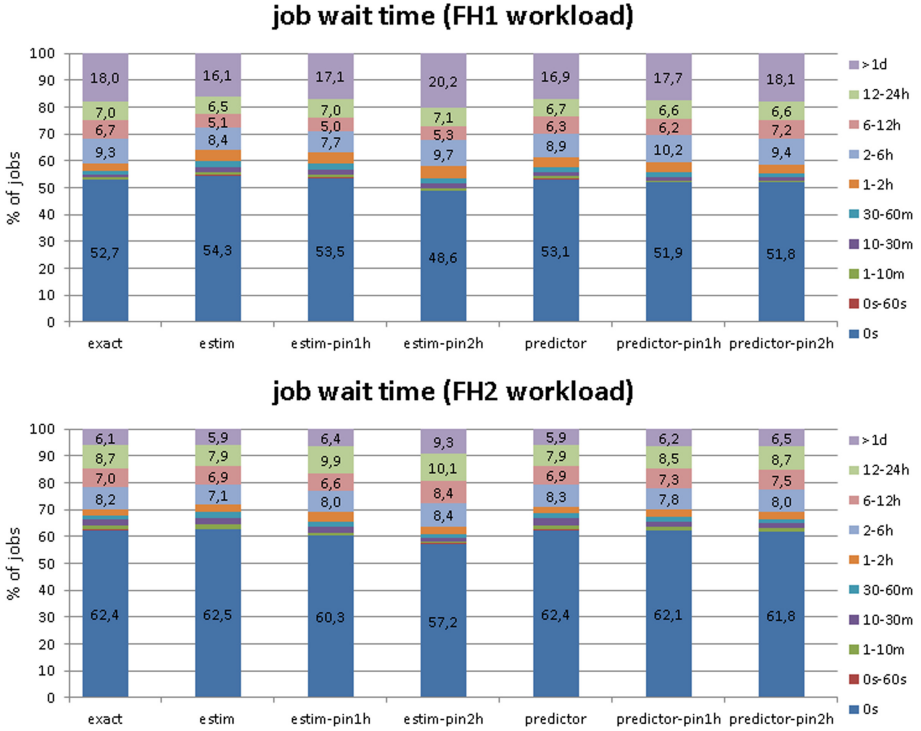
Fig. 13. Distribution of job wait times with respect to the pinning interval and walltime being used.
