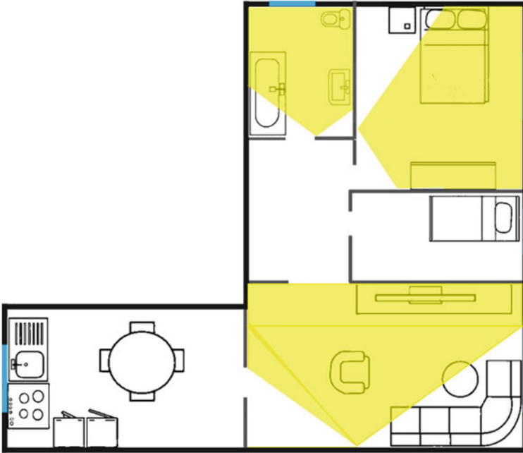
Fig. 2 Plan of the apartment and location of the 3 PIR sensors (placed in the living room, bathroom and the bedroom, respectively)
