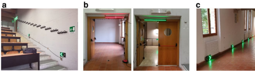
Fig. 4 View of the Co-WayS application in the testing scenario: a stepped classroom (directional sign and, on the top, the U_3 door sign); b door sign (prohibited access, red; to be used, green); c along the corridor (directional arrows)
