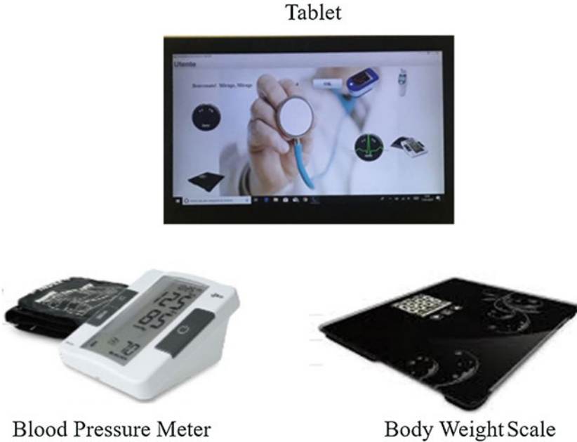
Fig. 1 The customized user interface for data collection, a blood pressure meter to monitor the blood pressure and heart rate and a body weight balance to acquire the body weight
