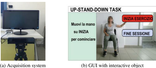
Fig. 1 a The vision-based system consisting of RGB-Depth camera, mini-PC and monitor. b Example of GUI with interactive objects to perform selections
