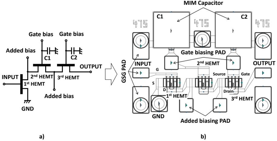
**Fig. 1.** Proposed 3-stacked GaN HEMT topology: a) Schematic and b) MMIC layout.
