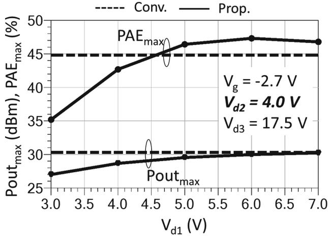
**Fig. 4.** Maximum PAE and Pout as a function of varied  $V_{d1}$ . Performance comparison with a conventional structure is also shown.
