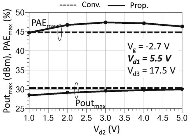
**Fig. 6.** Maximum PAE and  $P_{out_{max}}$  as a function of varied  $V_{d2}$ . Performance comparison with a conventional structure is also shown.
