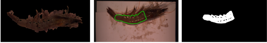
Fig. 3. Preprocessing and extracting data of shrimp from hyperspectral image. (a) our first mask which removes white noise and white background. (b) boundary of shrimp body after using Labelme. (c) the last mask achieved by combining our first mask (a) and boundary (b)
