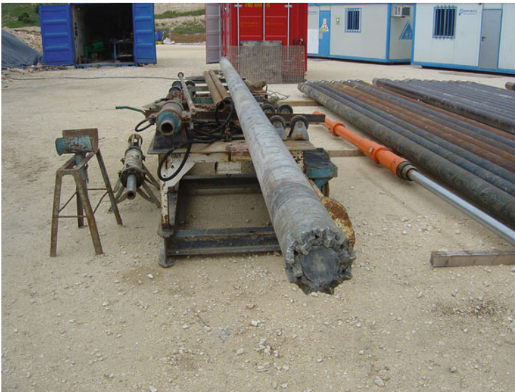
Fig. 10 Drilling tool and pipe for coring used at Hontomín (Courtesy of CIUDEN)
