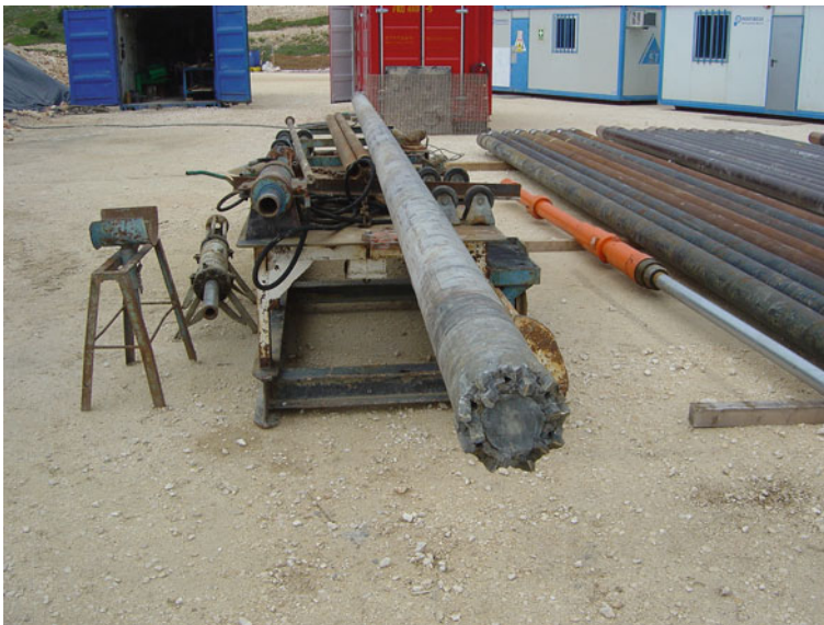
Fig. 10 Drilling tool and pipe for coring used at Hontomín (Courtesy of CIUDEN)
