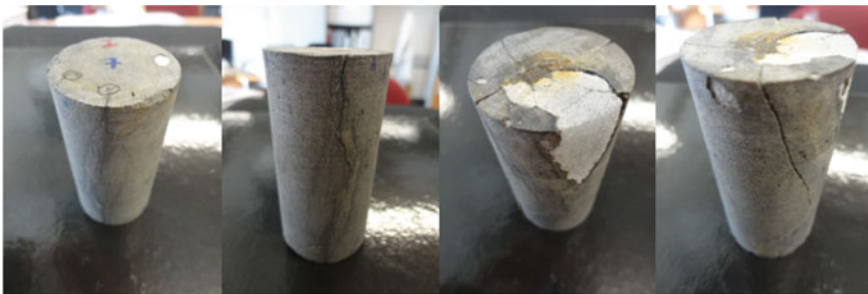
Fig. 19 Injection (left) and production (right) surfaces of the plug after co-injection
