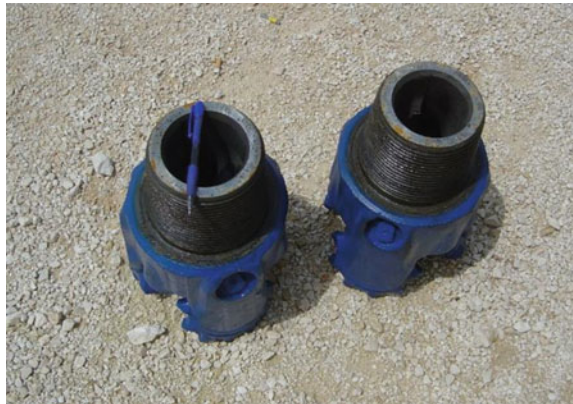
Fig. 8 Drilling bits used at Hontomín (Courtesy of CIUDEN)
