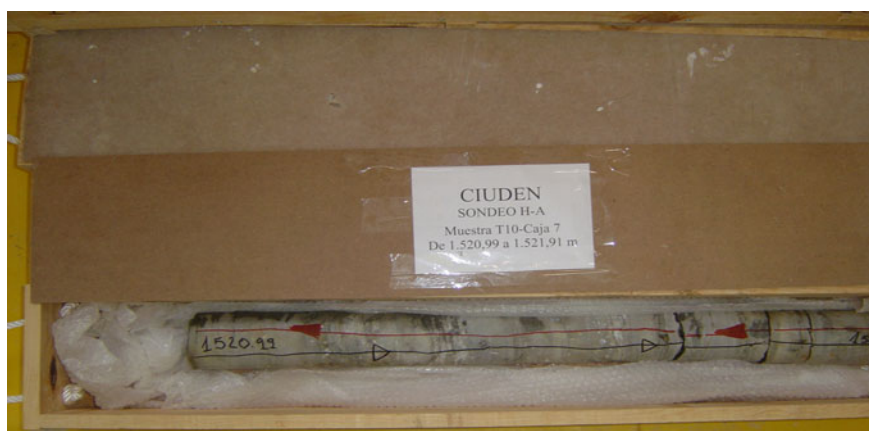
Fig. 3 HA sample 10 (drilling interval: 1515–1522 m) (Courtesy of CIUDEN)
