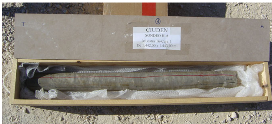
Fig. 11 Core sample from limestone Sopeña Formation in the observation well (Courtesy of CIUDEN)
