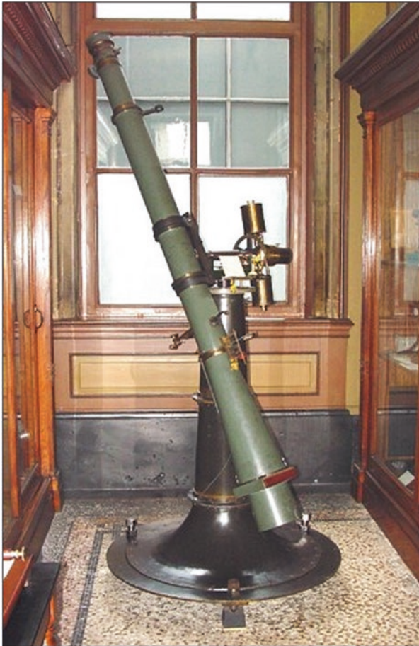
Fig. 7.16 The Dallmeyer photoheliograph that was taken to Réunion for the 1874 transit of Venus ( http://www.mi-aime-a-ou.com/photo_la_reunion.php?id_img=5326 ).
