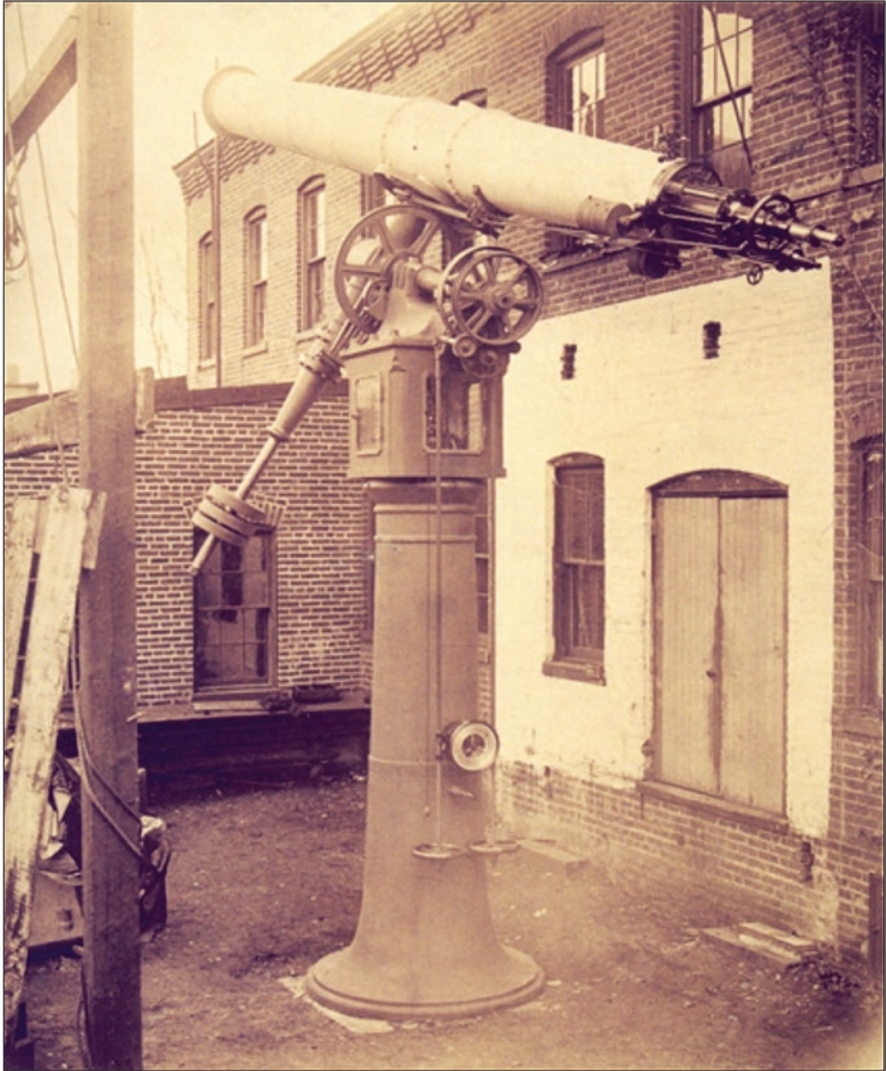
Fig. 1.16 A photograph of the 19-in refractor destined for Manila Observatory mounted and operational in a builder's yard in Washington, D.C., USA (photograph courtesy: Patrick Seitzer).
