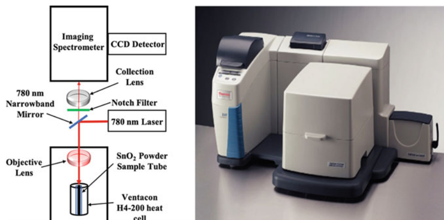
Fig. 2 Schematic of the Raman SmartDXR™ Spectrometer (left) and the Raman SmartDXR™ instrument (right). (Adapted from Casimir et al. [8])
