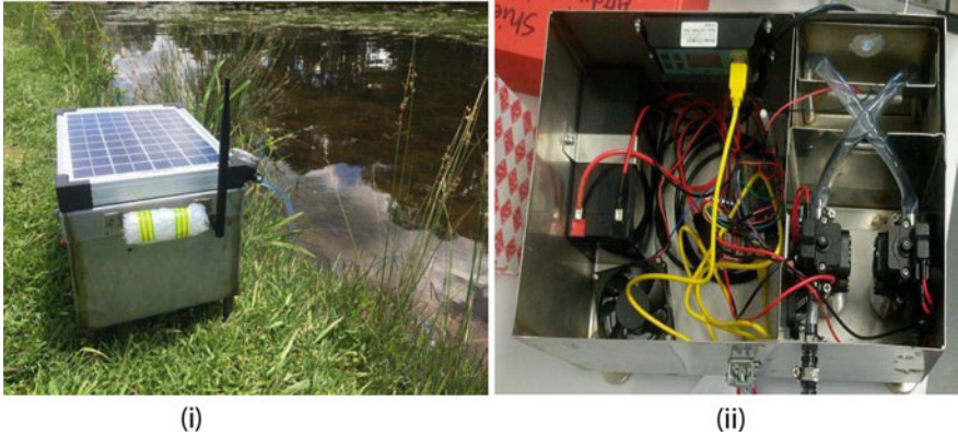
Fig. 13 IoT enabled interdigital sensor based nitrate monitoring; (i) the complete system; (ii) inside electronic components [31]
