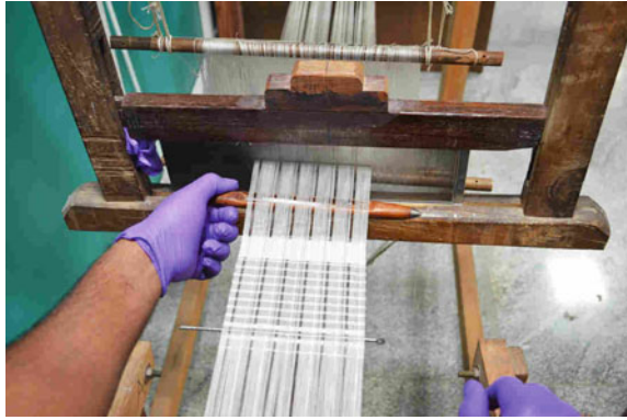
Fig. 11 A handloom used to weave silk strips, which would be used as glucose sensors [81]
