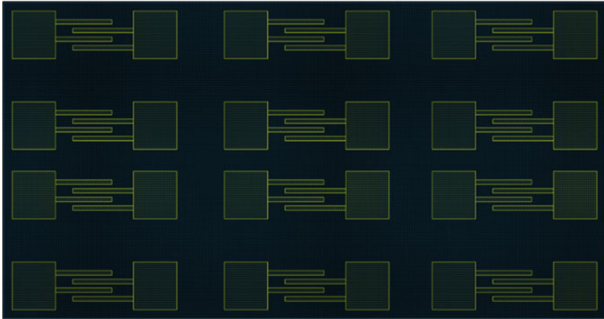
Fig. 11 The source-drain and IDC mask designed using the layout editor
