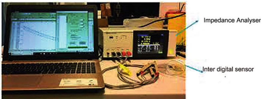
Fig. 5 A typical Impedance analyzer (Hioki LCR meter IM3536) [8]
