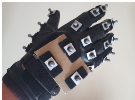
Fig. 7. A glove attached with 19 markers for tracking with optical motion capture systems. The three markers on the back of the hand have a fixed distance and can be interpreted as a rigid body.
