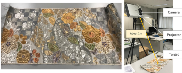
Fig. 4. Nishijin textile to be measured (left) and Experimental setup (right)
