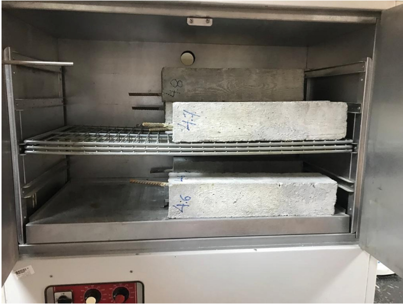
Fig. 9. Samples placed on an oven and subjected to 70 °C heating cycles
