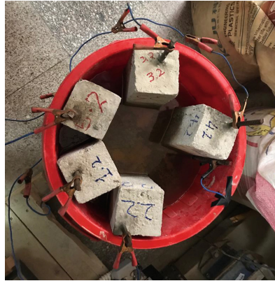
Fig. 5. Connected circuit for accelerated corrosion
