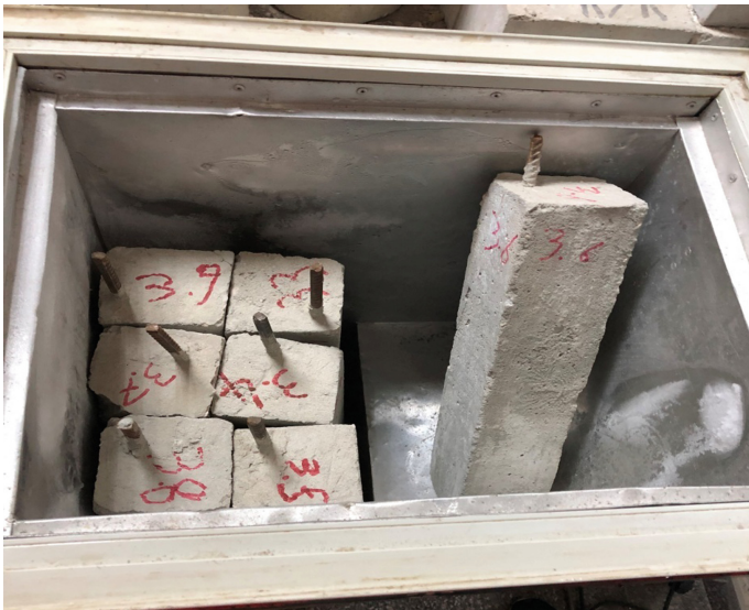
Fig. 8. Samples placed on a deep freezer and subjected to -2\text{ }^{\circ}\text{C} freezing and thawing cycles
