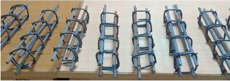
Fig. 2. Reinforcement steel cage
