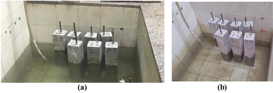
Fig. 7. Samples subjected to saltwater wet-dry cycles with water level is set to (a) 2/3 of column height for 3 days and 1/3 of column height for 4 days
