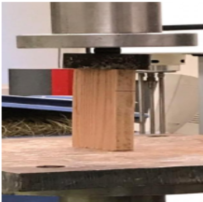
a. Testing for compression parallel to the grains
