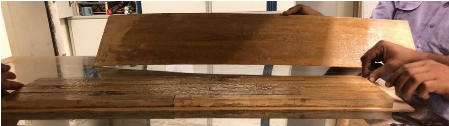
Fig. 2. The sandwicing of wood in between the two veneer layers.
