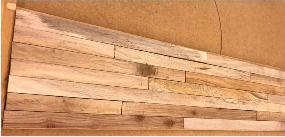
Fig. 1. The arrangement of wood within a blockboard panel.
