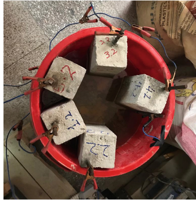
Fig. 5. Connected circuit for accelerated corrosion
