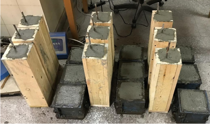
Fig. 4. Casted reinforcement concrete (RC) samples
