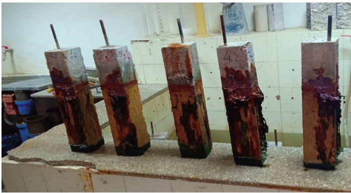
Fig. 6. Accumulated rust on the surface of the columns after accelerated corrosion
