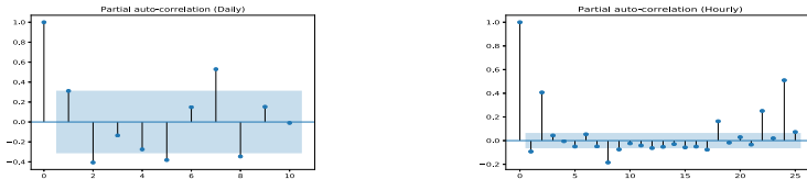
Fig. 4. The partial auto-correlations for the process arrival rate. Daily (left) and hourly (right) time windows (left).
