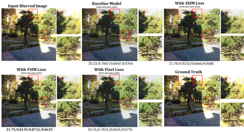
Fig. 2. Results generated by WGAN-GP model with different loss functions on GoPro dataset.
