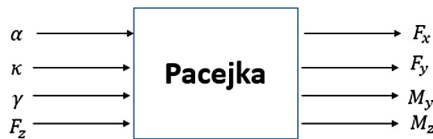
Fig. 2. Input and output of Pacejka Model
