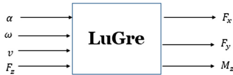
Fig. 12. Inputs and outputs of the LuGre model
