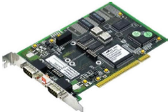
Fig. 3 PCI CAN-AC2 card used in the RT-Lab system for CAN bus communication
