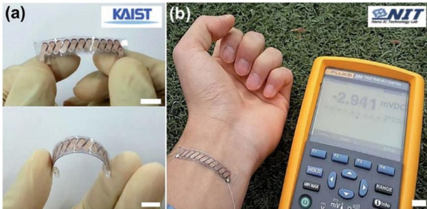
**Fig. 2** Demonstration of band-type flexible TE generator for harvesting thermal energy from human skin: (a) photos of band-type flexible TE generator and (b) electricity generation measured on human skin at an air temperature of 15 °C. Scale bar, 1 cm [12]
