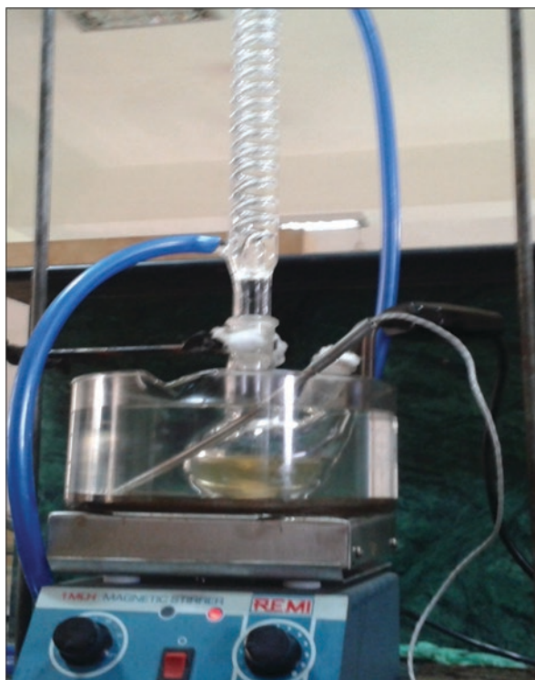
Fig. 18.2 Nanoemulsion preparation assembly
