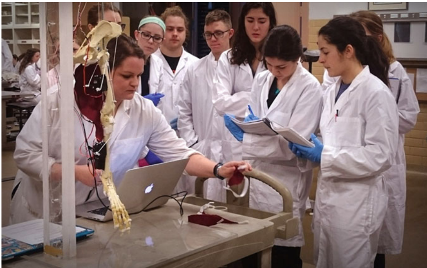
Fig. 18.3 Interactive Simulation Model being used in anatomy lab: This model utilized servo motors mounted to bones cast in plastic to create the actions of muscles in the canine pelvic limb. Students typed the name of a muscle into a computer and the simulation model would create the action of the specified muscle
