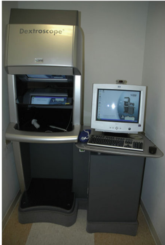
Fig. 16.7 Image of the Dextroscope VR system used in the study of Jang et al. (2017) to present inner ear structures to medical students. The student uses the system on the left side, whereas the right side is the interface for the teacher (From: Jang et al. 2017)
