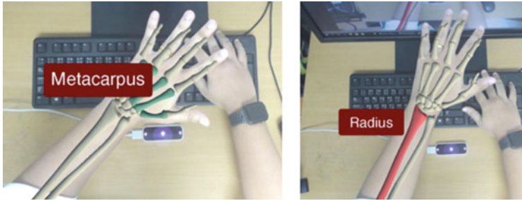
Fig. 16.6 Selected parts of the hand are labeled. Label placement is essential: the label on the left occludes part of the relevant image (From: Boonbrahm et al. 2018)
