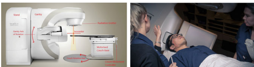
(a) An annotated image of a Varian TrueBeam LINAC machine [34].
