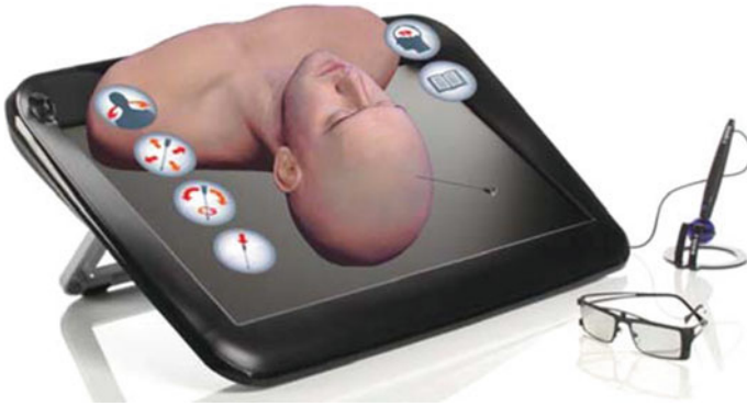
Fig. 16.8 The neurosurgery training application running on the zSpace presented by John et al. (2016) (artistic impression used in the figure to depict the 3D effect) (From: John et al. 2016)
