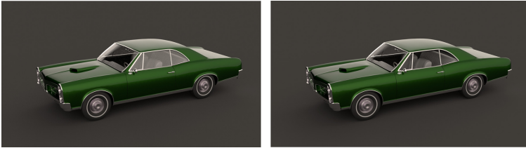
Fig. 4. Car [4] rendering without (left) and with (right) our four layers anti-reflective coating on the windows and the windshield. (Color figure online)
