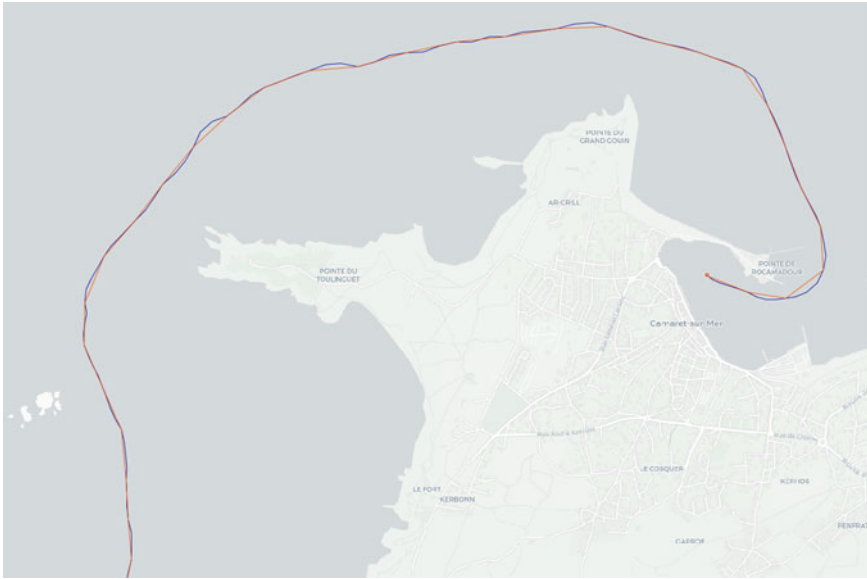
Fig. 4.9 Simplification example using the Douglas–Peucker method- in blue the original trajectory and in red the simplified version
