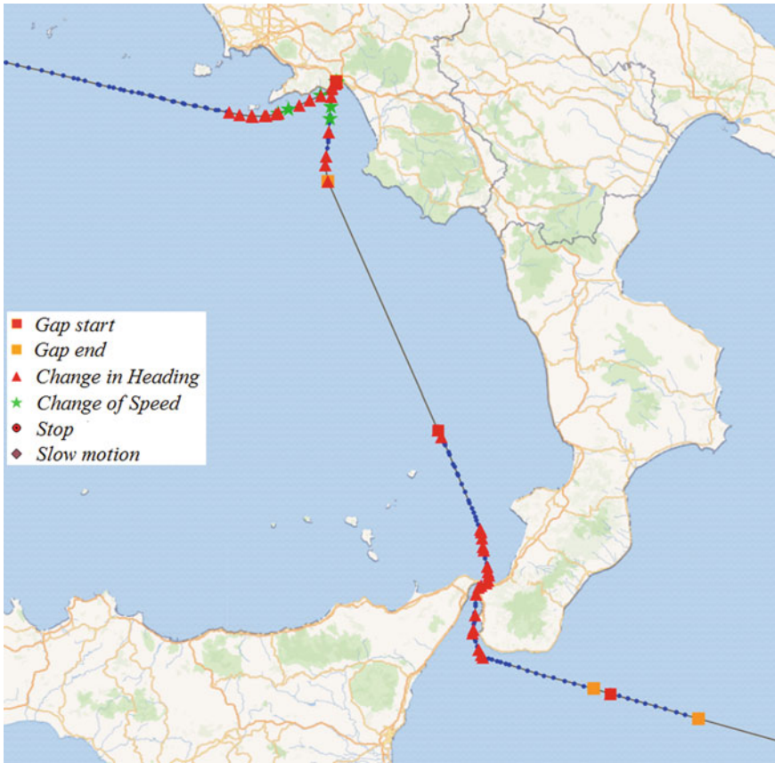
Fig. 6.1 Annotated critical points identified along a vessel trajectory. The sequence of such critical points provides a synopsis of the trajectory (shown as black line segments) with small deviation from the actual one. Original AIS positions not qualifying as critical are depicted in blue dots and generally concern straight segments of the vessel's course. Also note the lack of reported AIS locations (i.e., communication gaps) over large intervals along this vessel's route
