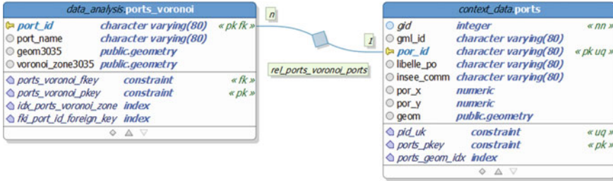
Fig. 3.15 Use of foreign keys to implement a one-to-many relation between ports and Voronoi tessellation (extracted from the PostgreSQL maritime database using pgModeler)
