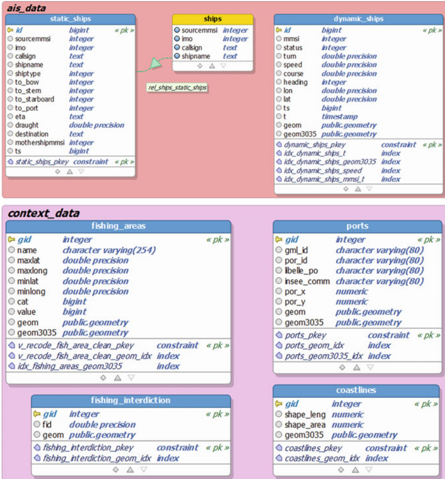
Fig. 3.13 Entities’ structure (tables and views) of the database schemas ais_data and context_data . The data model is extracted from the PostgreSQL maritime database using pgModeler
