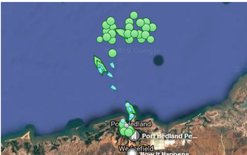
Fig. 11.1 Identification of anchorage and terminal polygons using AIS data. Source Marinetracfic.com/Google imagery
