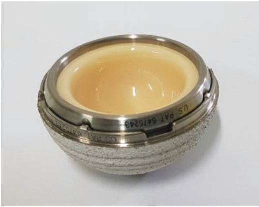
Fig. 13.3 Titanium-backed ceramic liner to prevent impingement between the stem neck and the ceramic liner rim
