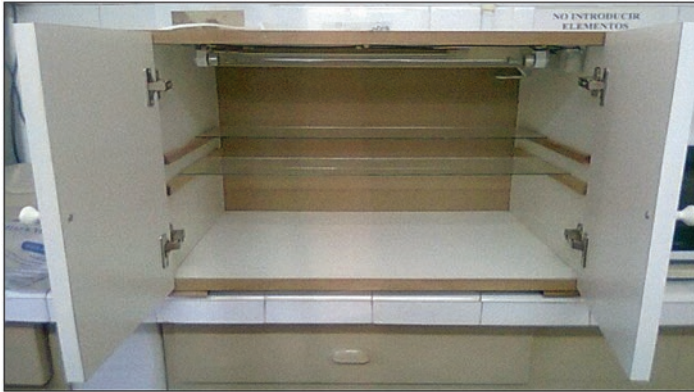
Fig. 2.1 Equipment designed for irradiated of meat samples with UVC light. In the top are the UVC light tubes
