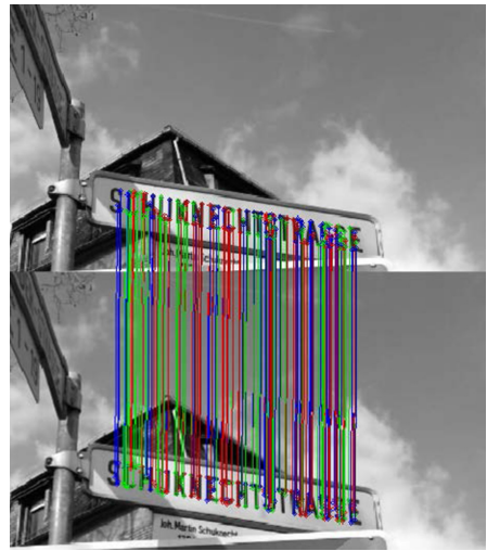
Fig. 7. Results of the multi-scale Lucas-Kanade algorithm on a street sign.
