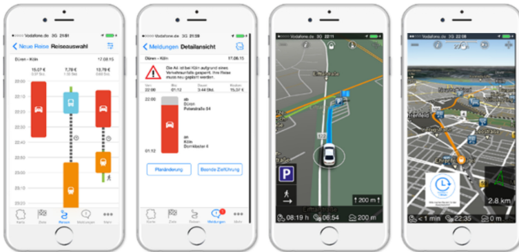
Fig. 5. The MoveBW smartphone application provides functions for intermodal journey planning, traffic information, ticketing and on-trip navigation. (Source: https://www.altoros.com/blog/mobile-devices-are-propelling-industrial-iiot-scenarios/ ).
