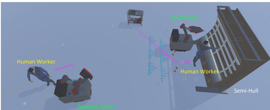
Fig. 11. Assembly scenario visualization in Unity3D.
