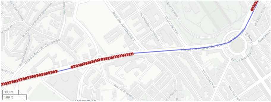
Fig. 4. Location detection issues inside of a tunnel.
