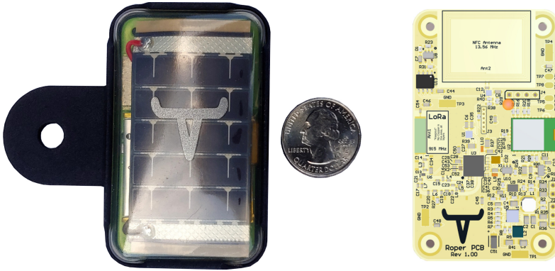
Fig. 1. (a) Roper cattle sensor in housing. (b) Graphic of the sensor board PCB.
