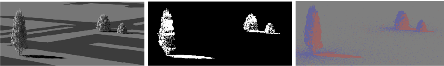
Fig. 4. Simulated DIRSIG scene with trees (left) and an occlusion and shadow mask ground truth image (center) showing all occluded and shadowed pixels in the scene in white, with spectral angle classification used to detect change between OSM terrain and the simulated image.
