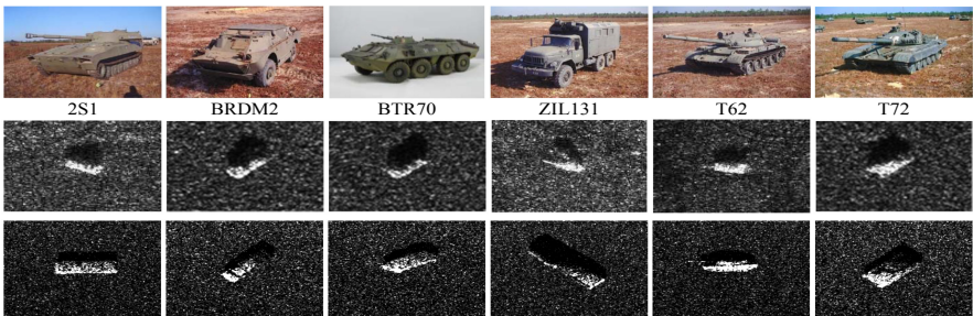
Fig. 3. Comparison of IRIS SRE method vs real SAR images from MSTAR dataset [7]. Top: sample military vehicles. middle: the corresponding vehicles' SAR image from MSTAR dataset. Bottom: simulated SAR image of the same vehicle models using our proposed IRIS-SRE method.
