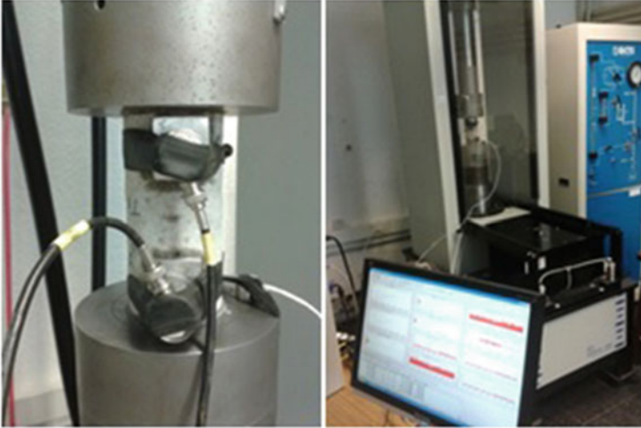
Fig. 1 The experimental setup and the AE system
