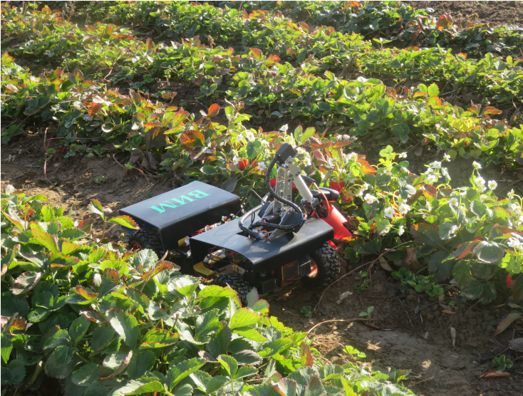
Fig. 6. Experimental model of an automated platform with a manipulator and a computer vision system
