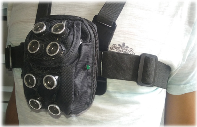
Fig. 1. BlinGui: electronic device to detect obstacles.
