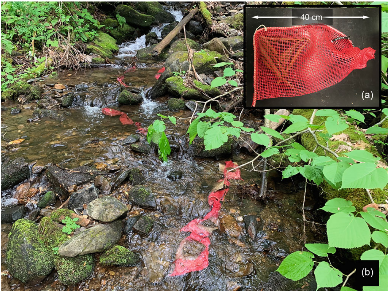
Fig. 7.7 Leaf litter bags deployed in a stream in the southeastern US. Each mesh bag contains the same quantity of previously dried and weighed leaves. Leaves are retrieved, dried, and re-weighed at
