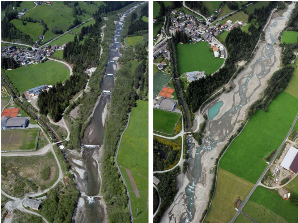
Fig. 15.4 Views of the Mareta River, Italy, before (left, 2005) and after (right, 2010) river restoration that removed grade-control structures. Source Archivio fotografico dell’Agenzia per la Protezione civile/Luca Messina–Provincia Autonoma di Bolzano
